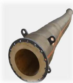
The Series 6000 is the flagship of the hose line with the best utility for most applications. This medium-duty hose is available in lengths from 5 to 50 feet and 3” to 40” ID. With excellent flexibility for discharge duty and light suction, this hose can handle up to 150 PSI operating pressure.
